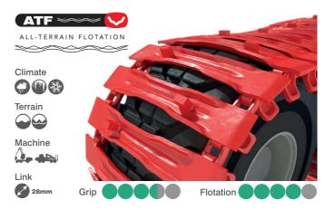
Designed for use in wet marshy conditions and also snow and ice. A special link system is utilised to enable better cleaning and ejection of snow and mud. Wide and upturned edges give flotation whilst a pinched mid-section generates traction.
